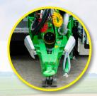
"V-shaped" drawbar housing the pump system
